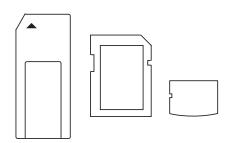
Figure 4-2. Memory Stick, Secure Digital, and xD Cards
